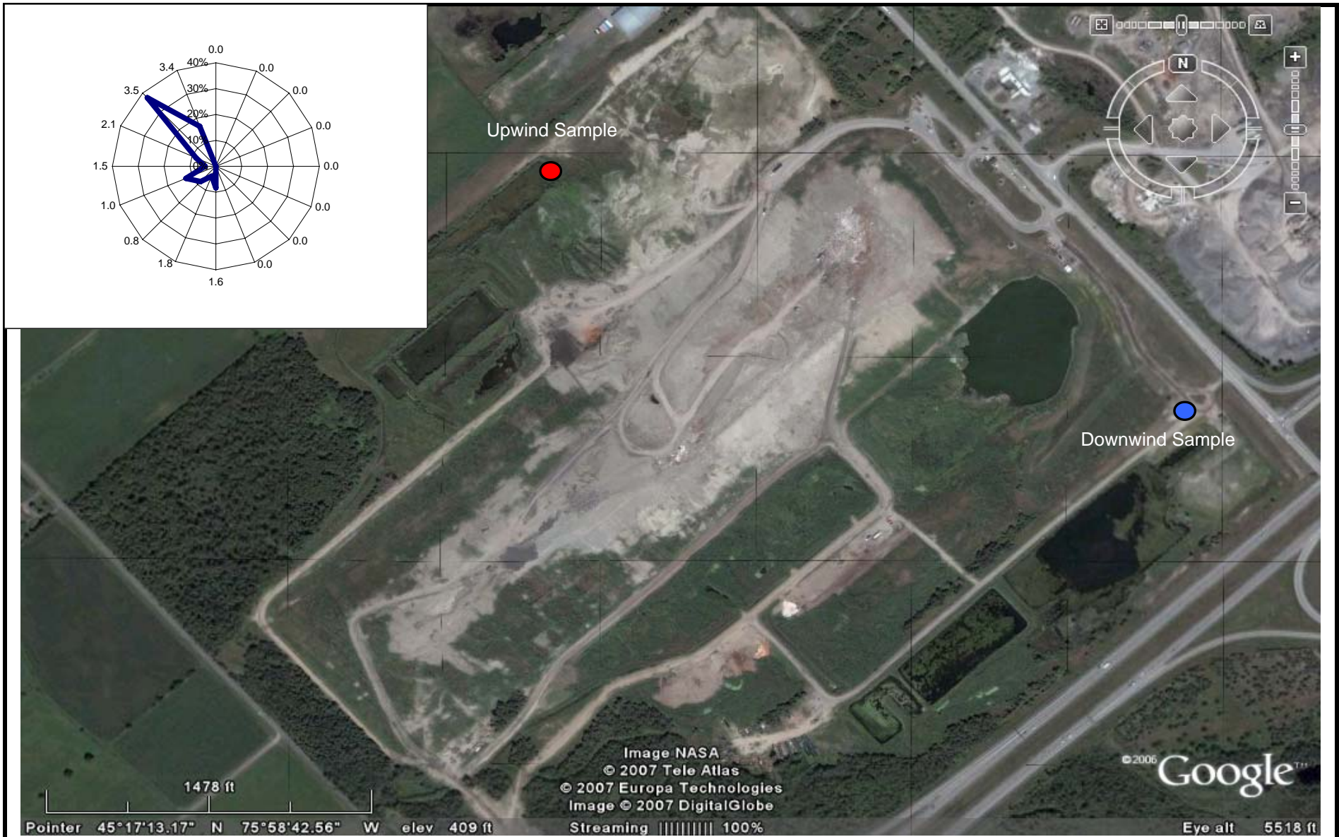
BTEX Sampling - Recommended Locations for June 23, 2008 Windrose from On-Site Meteorological Station Showing Winds Blowing From and Mean Wind Speeds
